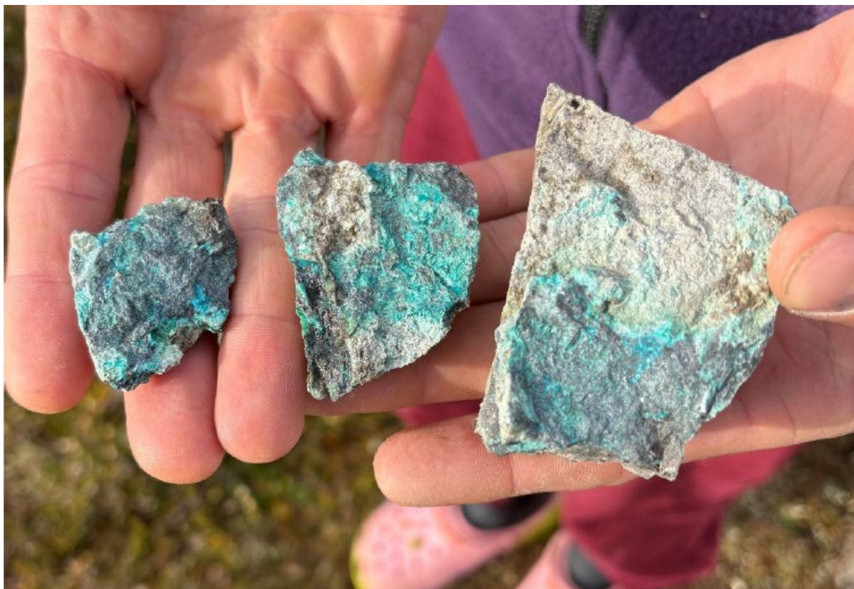
Figure 5. Misty Mtn Zone: Sample AOTHR044: chrysocolla and chalcocite in veinlets
