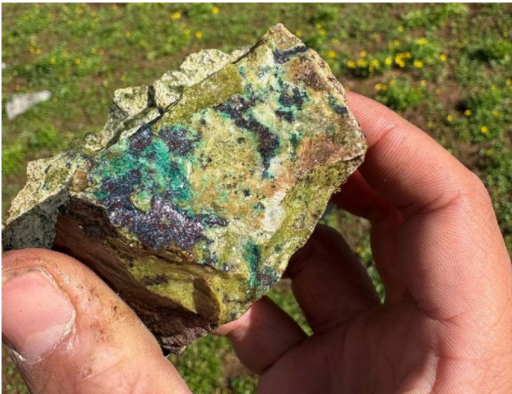
Figure 4. Rock Sample THTHR086: strongly epidote altered basaltic andesite with bornite, chalcocite and cuprite
